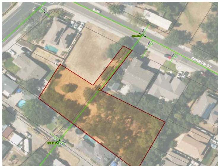
Existing 12-inch sewer trunk line.
