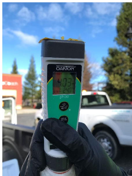
Figure 8 - 03/20/2023 - pH reading of 4.03.
