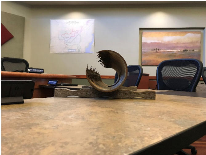
Photo 14 - 04/06/2023 - Severe deterioration from discharge that exceeds local limits.
