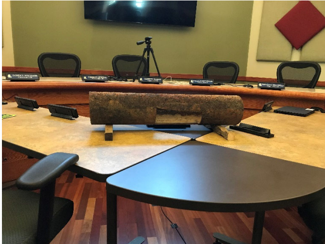
Photo 13 - 04/06/2023 - Pipe removed after retrieving stuck cleaning nozzle.
