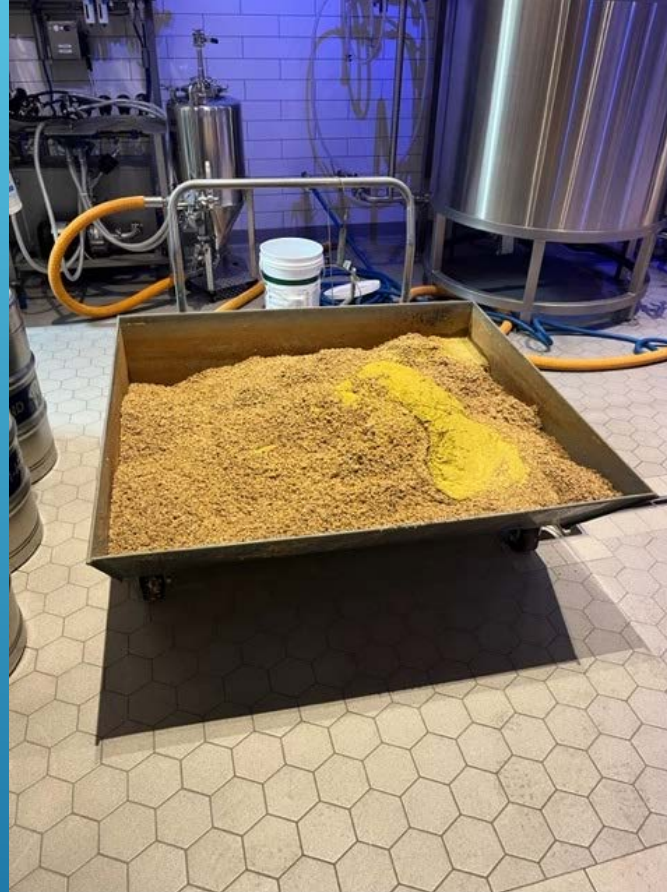
Brewery solid waste collection bin. All heavy solids are removed from their wastestreams.
